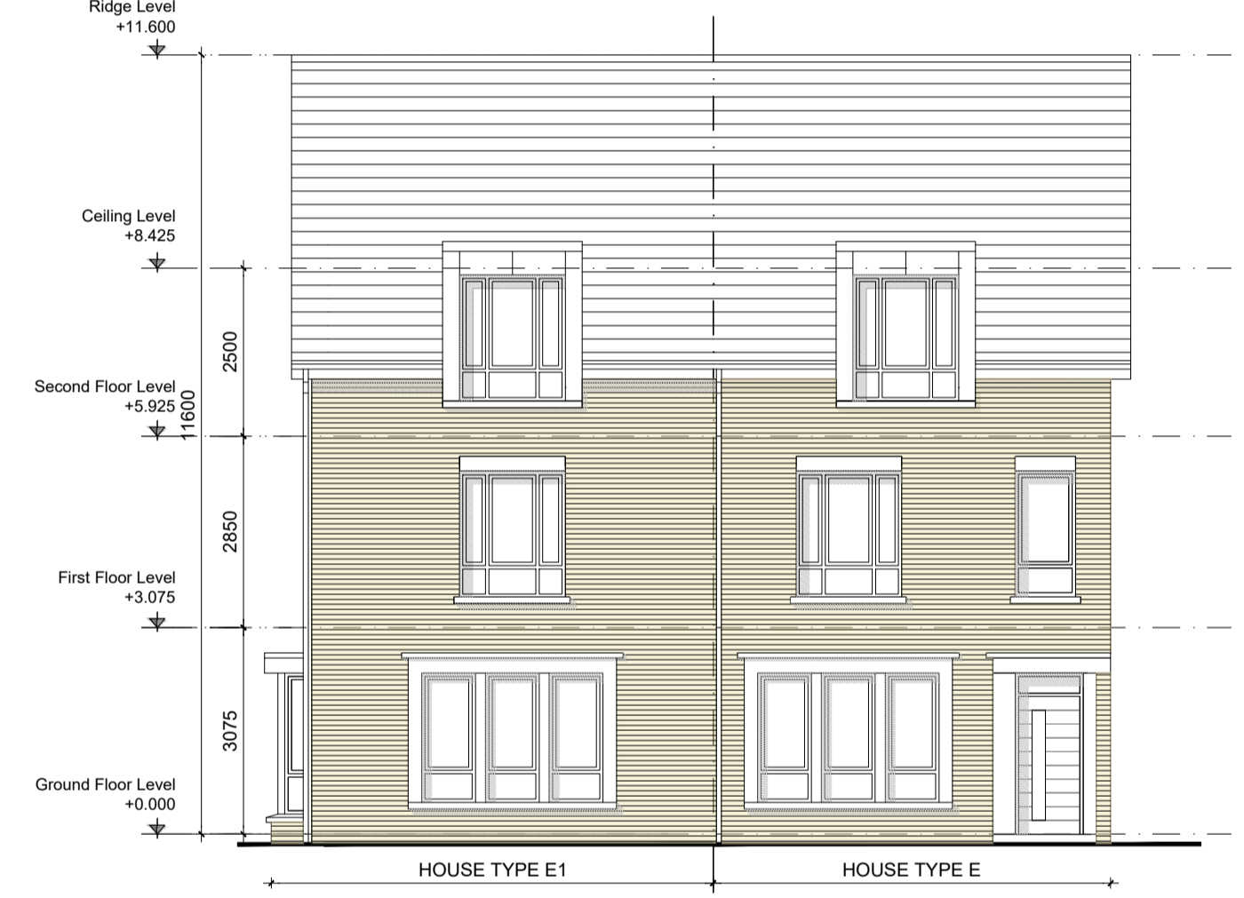
FRONT ELEVATION - CHARACTER AREA 1 (Buff Brick)
